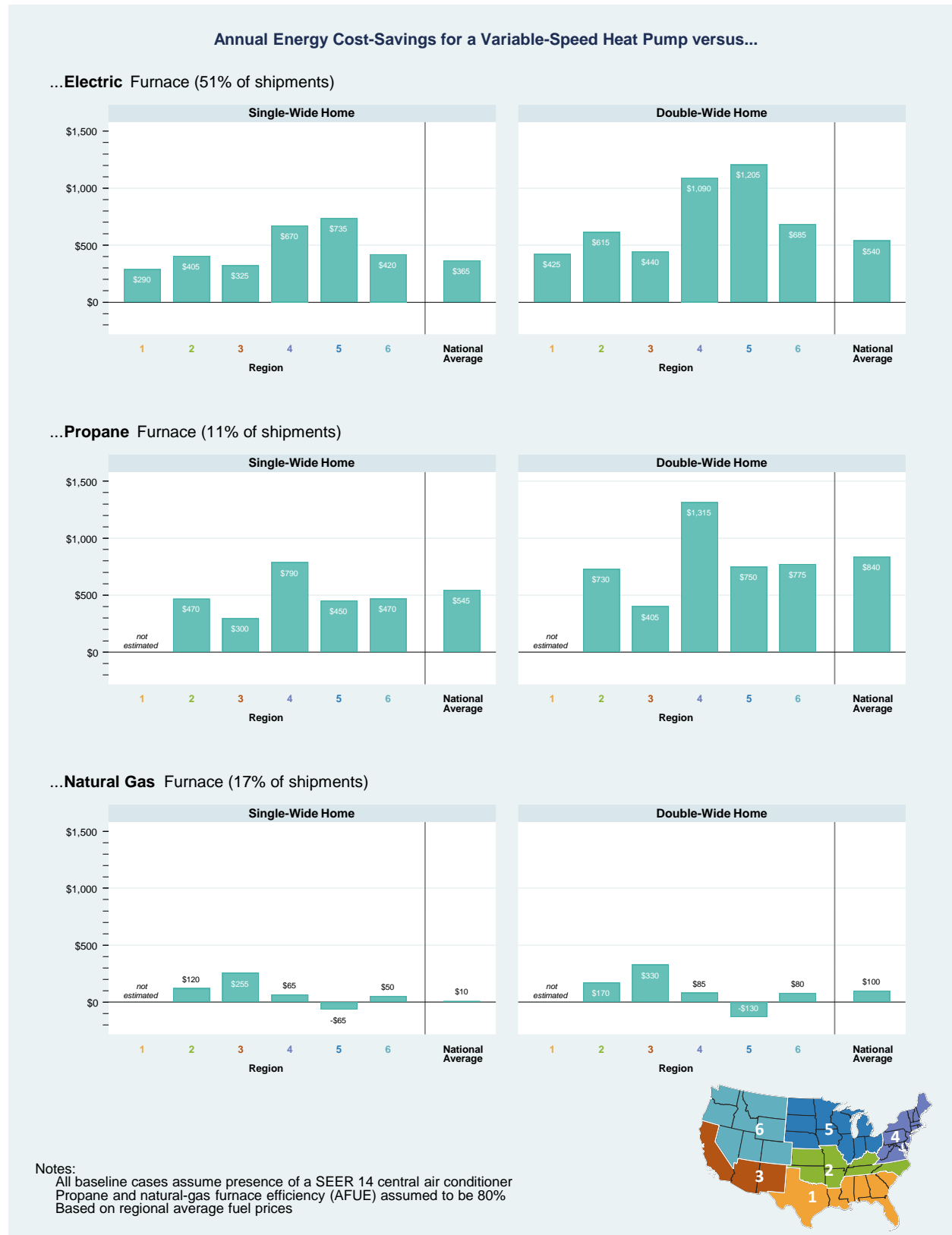
Figure 17. Annual energy-cost savings for a variable-speed heat pump versus a furnace and central air conditioner, by furnace fuel, home type and region.
