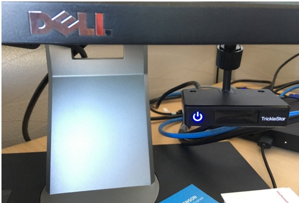
Figure 3: Device B occupancy sensor connected mounted to monitor and connected (via USB) to laptop.
