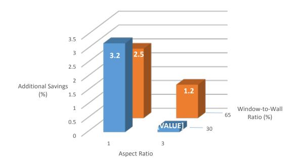
For the APS, the average additional HVAC savings was 1.8%, which was three percentage points less than that of CPM. This is because the APS saves most of its energy at night and on the weekends, and there are relatively higher heating loads in an office at night (in Minnesota) than there are during the day. The same significant impact is seen for the variance in aspect ratio. With the APS scenarios though, there is greater impact from changes in window-to-wall ratios as well.
