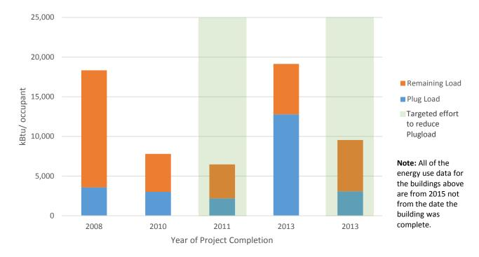
Figure 55. Single company across different sites – a case for plug load reduction.
