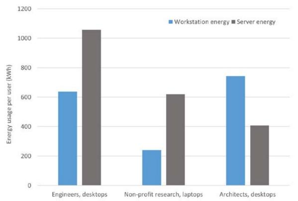
Figure 56. Office energy usage per workstation for the energy used at the workstation as well as that used in the server room.
