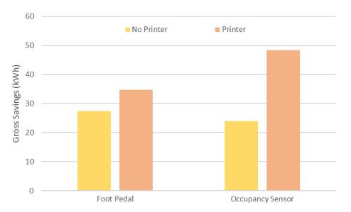
With the occupancy sensor APS, there was a substantial increase in the energy saved when a printer was present. If building owners or operators are conducting a more targeted campaign against plug loads, they could consider targeting workstations with larger extra devices – like printers – first.
