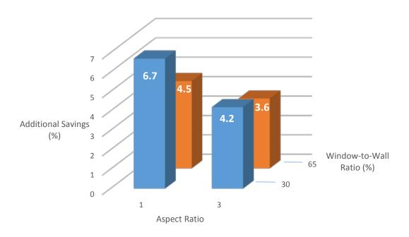
For these four scenarios, the average additional HVAC savings for CPM was 4.8%. The scenarios with an aspect ratio of 1 had significantly greater HVAC savings, because a building with a low aspect ratio has a large core space that is *always* in cooling – plug load reduction is always saving additional cooling energy in that space.
