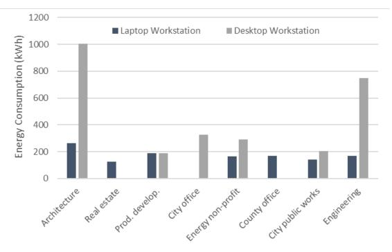
Figure 21. Baseline workstation consumption of desktop and laptop workstations.
