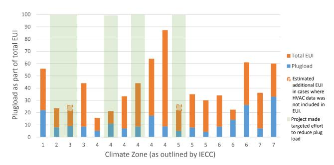
Figure 54. Plug load energy use intensity based on climate zone.
