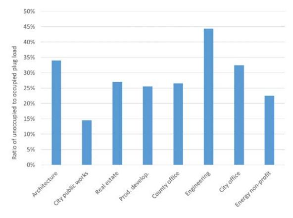
Figure 24. Ratio of the average unoccupied plug load to the average peak occupied plug load, for each office.
