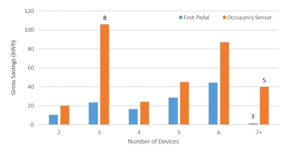
Figure 36. Gross savings versus number of devices sorted by foot pedal or occupancy sensor measures. Numbers above bars represent sample size, where the sample was small.
