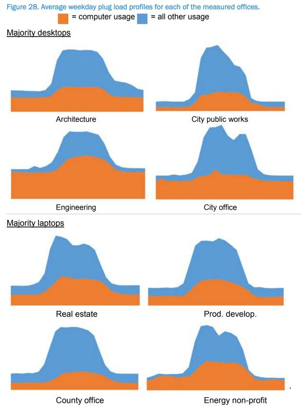
The Architecture site has a low average EFLH, likely driven by short periods of time doing very computationally intensive work that is not sustained much of the year. Conversely, the City office site has steady, moderate computer usage and therefore a higher EFLH. These usage
