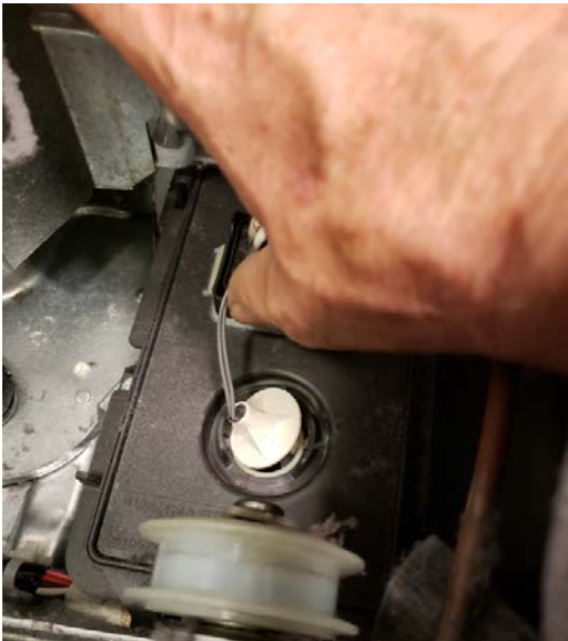
Figure 17, Partially-seated float switch for the malfunctioning heat pump dryer at Site 1.
