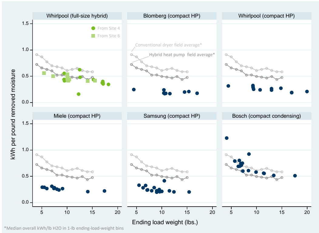
Figure 19. Energy performance versus load weight, comparing bench-testing results and field-monitoring averages.
