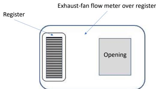
Figure 18. Modification to exhaust-fan flow meter for multiple pressure taps inside the meter.
