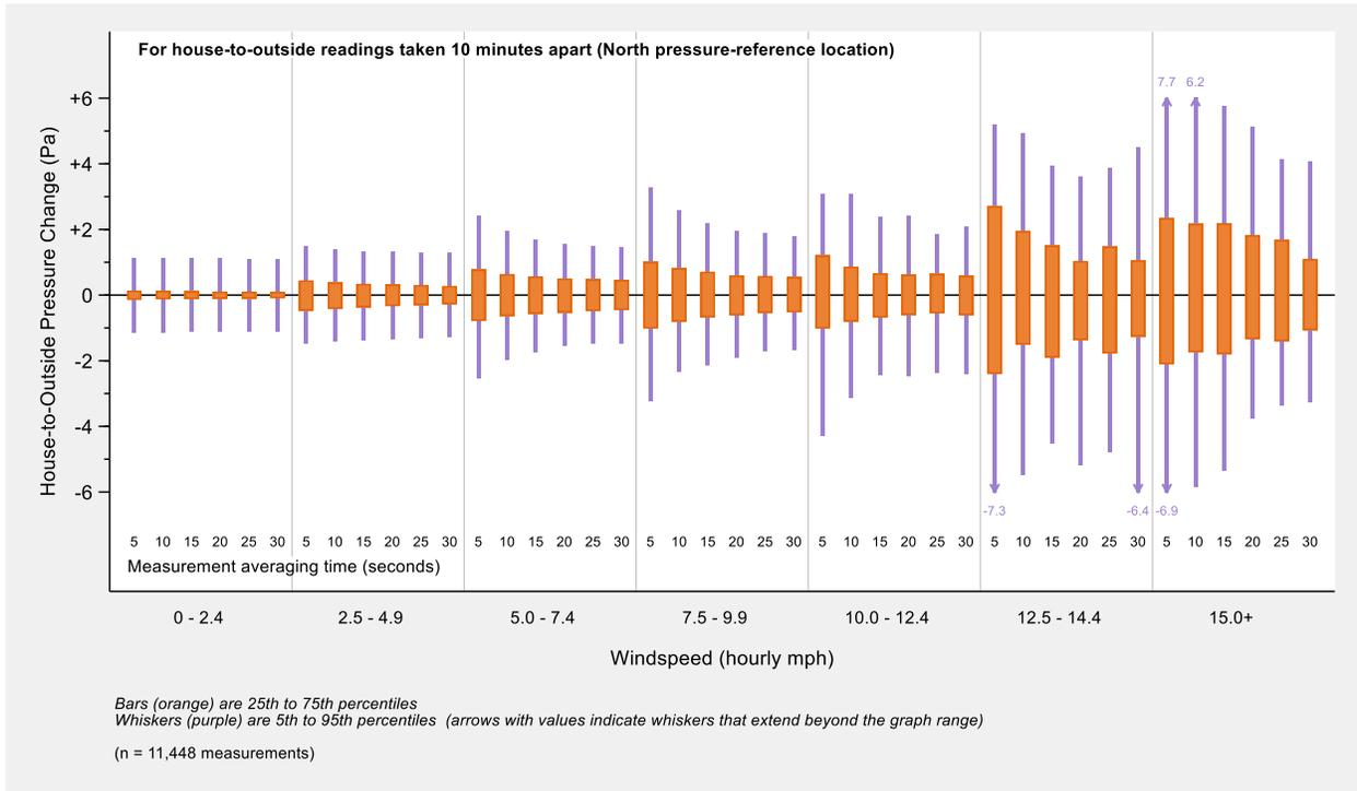
Figure 26. Distribution of baseline house-to-outside pressure variability at the FSEC MH Lab home, by measurement interval and windspeed.
