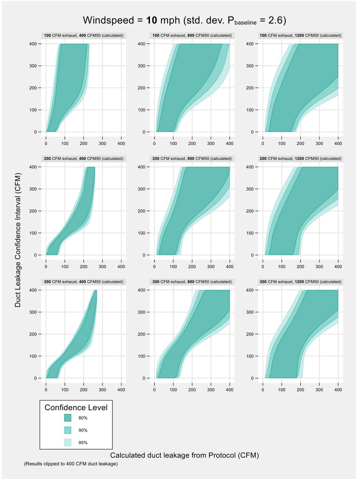
Figure 43. Confidence intervals for protocol-calculated duct leakage vs. observed house depressurization during air-handler operation, for selected levels of observed house depressurization during exhaust operation and windspeed, for 150 cfm of rated (but unmeasured) exhaust flow.
