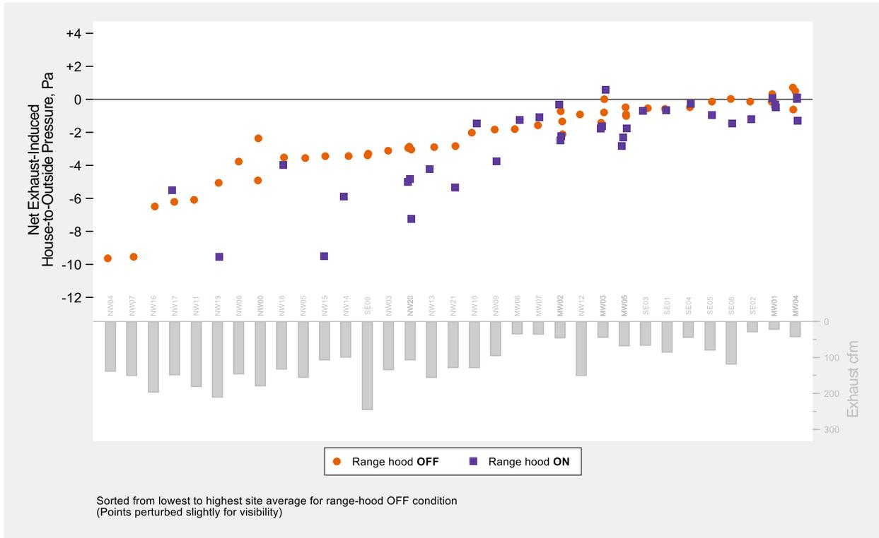
Figure 14. Baseline-adjusted house-to-outside pressure during air-handler operation.
