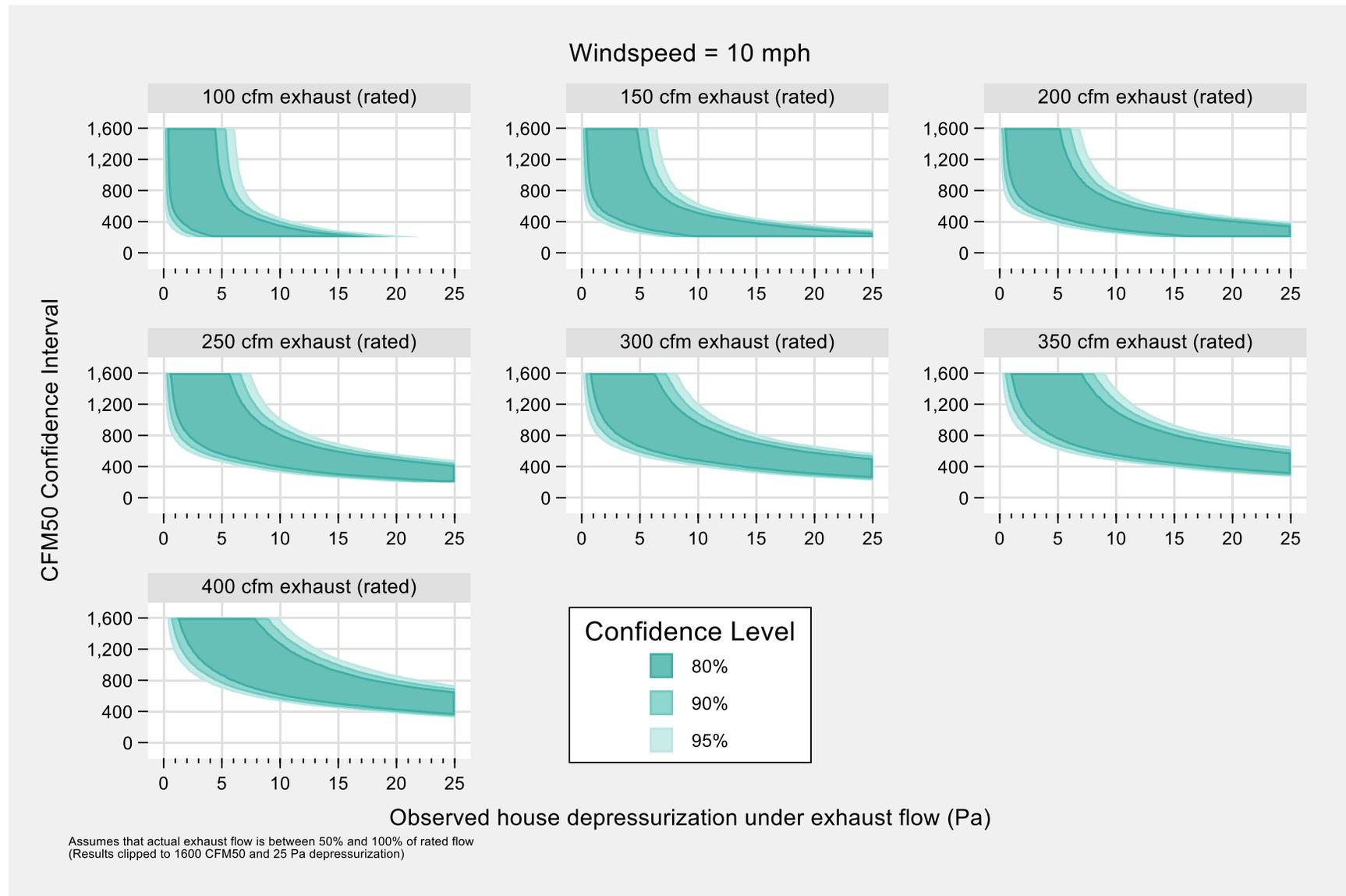
Figure 40. Confidence intervals for protocol-calculated duct leakage with measured exhaust flow, for selected exhaust-flow and protocol-calculated envelope leakage levels, 1-mph wind.
