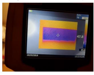
Figure 20. Uninsulated attic hatch (Site 183).
