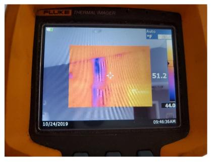
Figure 22. Example of a wall-insulation coverage issue (Site 182).
