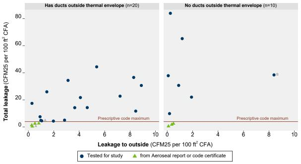
CFM25 = Cubic feet per minute @ 25 Pa pressure difference CFA = Conditioned floor area (Leakage to outside estimated for Aeroseal cases)
