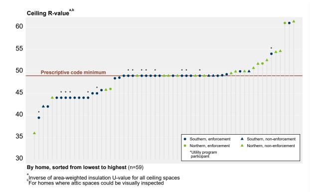
Figure 19. Distribution of ceiling R-value for homes where ceiling insulation could be visually inspected.
