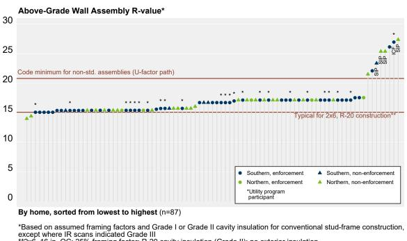
$x^{*2}x6$ , 16 in OC; 25% framing factor; R-20 cavity insulation (Grade II); no exterior insulation SIP = structural insulated panel; ICF = insulated concrete form
