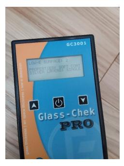
Low-e coatings are produced in two fundamentally different ways: hard (pyrolytic) coatings and soft (sputtered) coatings. The former has higher solar heat gain than the latter. Soft-coat low-e glazing can further be distinguished by the number of applied "silver" coatings, with solar heat gain declining as the number of coatings increases.
