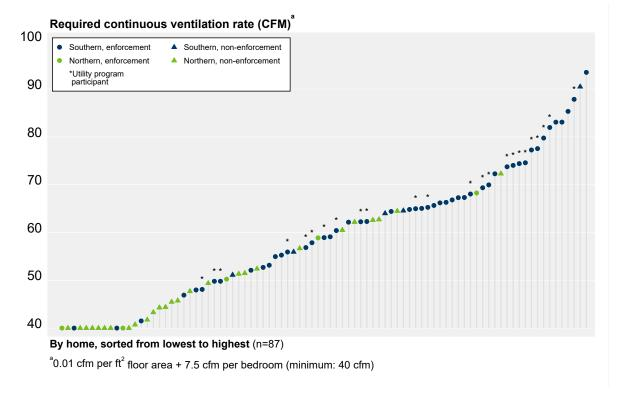
Figure 35. Required continuous ventilation rate.
