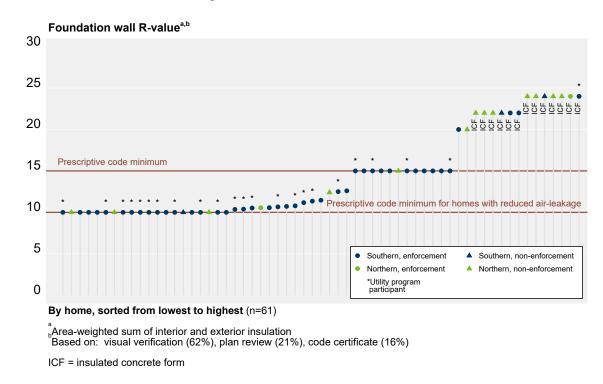
As shown in Figure 24, foundation wall insulation in the sample generally falls into three clusters: about R-10, R-15 and R-20 and higher. The first mostly comprises homes that meet the air-leakage requirements for reduced (R-10) foundation insulation. The second comprises homes that match the prescriptive energy code requirement. The third is almost entirely homes with ICF foundation walls.
