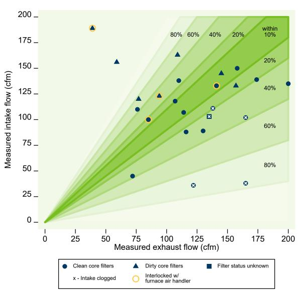
Figure 39. Measured HRV/ERV intake versus exhaust flow (n=24).
