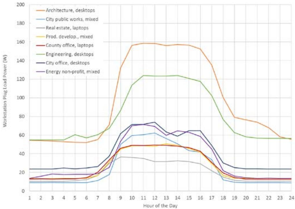
Figure 23. Workstation energy usage in a typical weekend day for each office.
