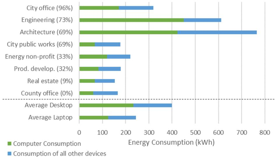
Figure 20 also shows the impact of desktops versus laptops on computer energy usage. The percentage of each site that used desktop computers is shown in parenthesis (e.g. 96%). The average energy usage of all desktops and all laptops respectively is also shown at the bottom of the figure. Workstations with desktops of course use more energy than those with laptops, and a significantly higher fraction of the energy used at workstations with desktops is used by computers.
