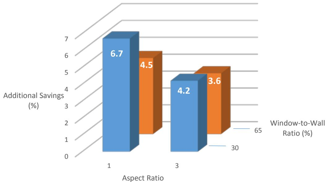
For these four scenarios, the average additional HVAC savings for CPM was 4.8%. The scenarios with an aspect ratio of 1 had significantly greater HVAC savings, because a building with a low aspect ratio has a large core space that is *always* in cooling – plug load reduction is always saving additional cooling energy in that space.
