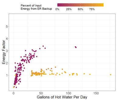
Figure 13. Daily energy factor by daily water consumption for site 06, with colors scaled to the percent of input energy from electric resistance backup.
