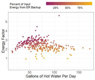
Figure 14. Daily energy factor by daily water consumption for site 03, with colors scaled to the percent of input energy from electric resistance backup.
