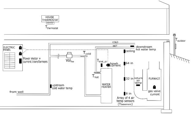
Figure 3. Monitoring system component positions.
