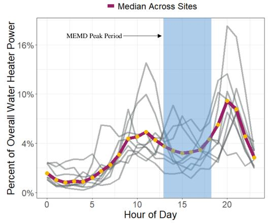
Figure 28. Hourly loads by site (in grey) and median across sites. Shading shows the MEMD-defined coincident peak period.<sup>31</sup>
