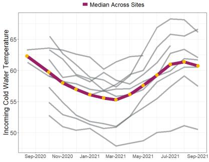
Figure 9. Average monthly incoming cold water temperature by site over the monitoring period. Hot and cold water temperatures are weighted by flow.
