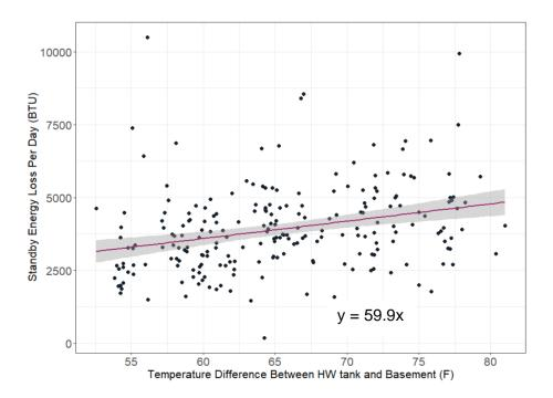
Figure 15. Standby loss vs tank - basement temperature difference for all sites, with regression line.
