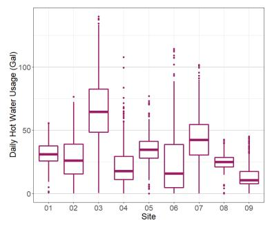
Figure 7. Distribution of daily hot water use by site. The boxes represent the 25<sup>th</sup> to 75<sup>th</sup> percentiles, and the heavy line is the median value. For readability, plots exclude the highest one percent of observations. Days of no hot water use are included.
