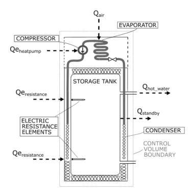
Figure 5. Energy entering and leaving a heat pump water heater, with control volume.
