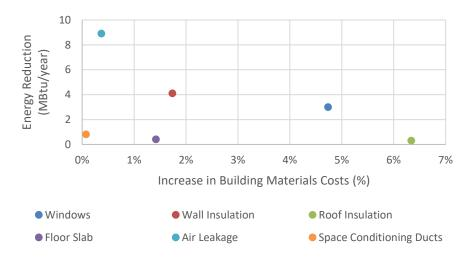
Figure 4. Building envelope upgrades from IECC 2009 to 2021 – energy and cost comparison
