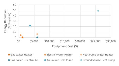
Figure 5. Building HVAC and water heater upgrades – energy and cost comparison
