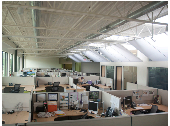
Figure 2: Seventhwave's skylight and baffle design
