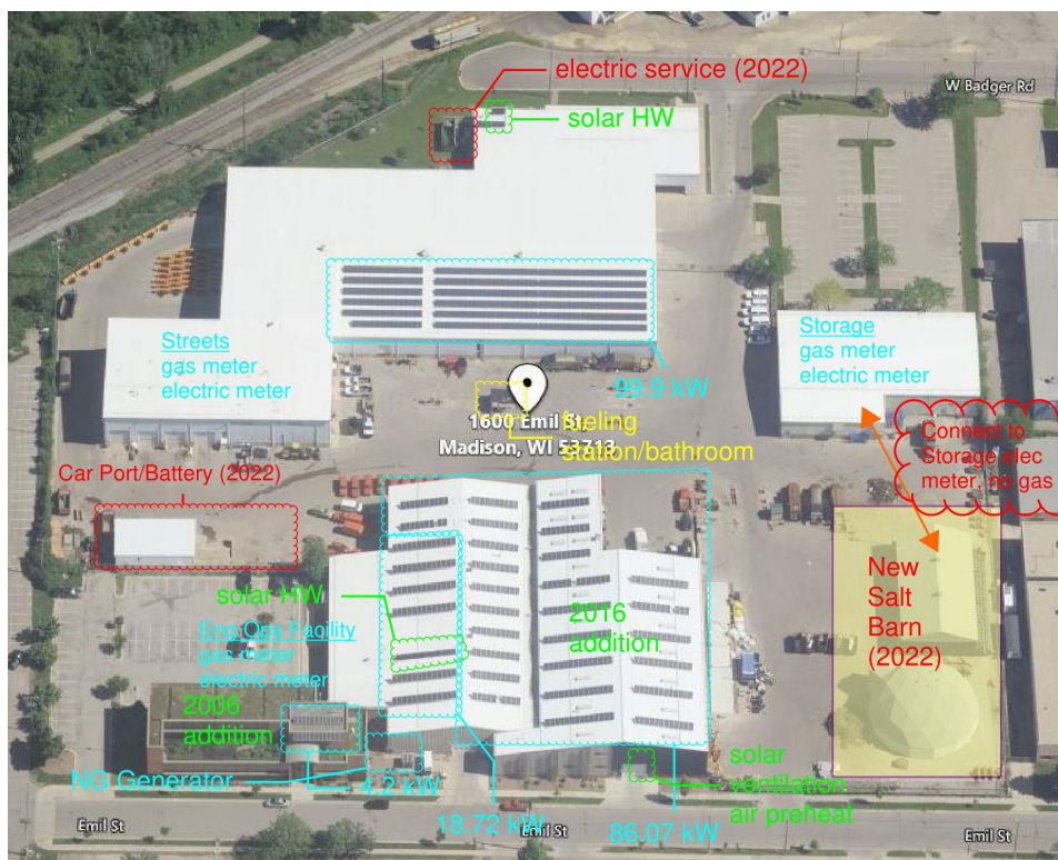
Figure 1. Site layout for Streets West (north/top of image) and Engineering Operations (south/bottom of image) showing proposed changes. PV array shown in Streets West rooftop is the initial 99 kW array; the additional 200 kW array was installed after this photo was taken.
