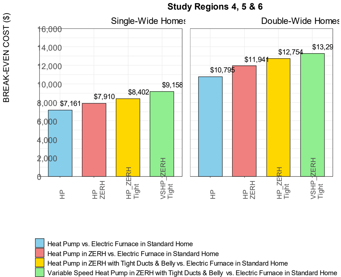
Figure 38. Incremental first cost at which a measure is a good choice from a consumer cost-savings perspective. Weighted average of regions 4, 5 and 6 (cold climates).
