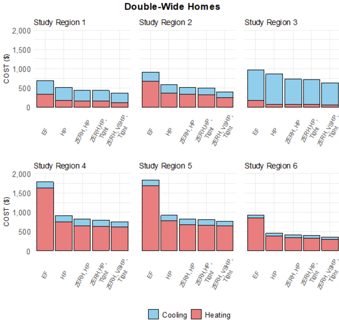
Figure 31. Weighted regional average heating and cooling costs of baseline envelope with various systems, for double-wide homes.
