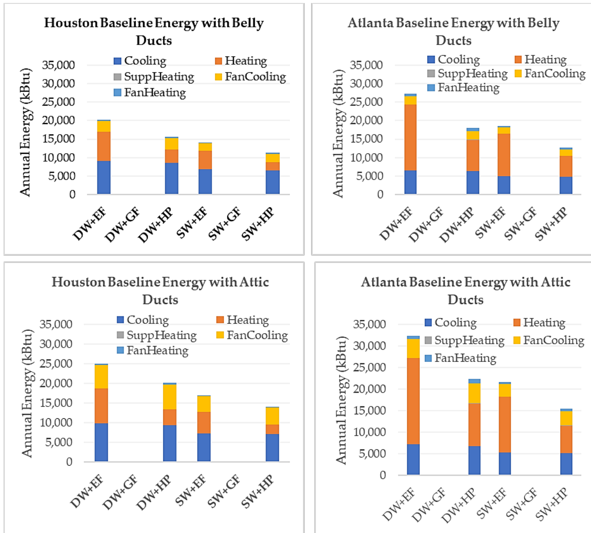
Figure 9. Baseline energy use with belly and attic ducts in Houston and Atlanta, for double-wide (DW) and single-wide (SW) prototype homes, by HVAC type.
