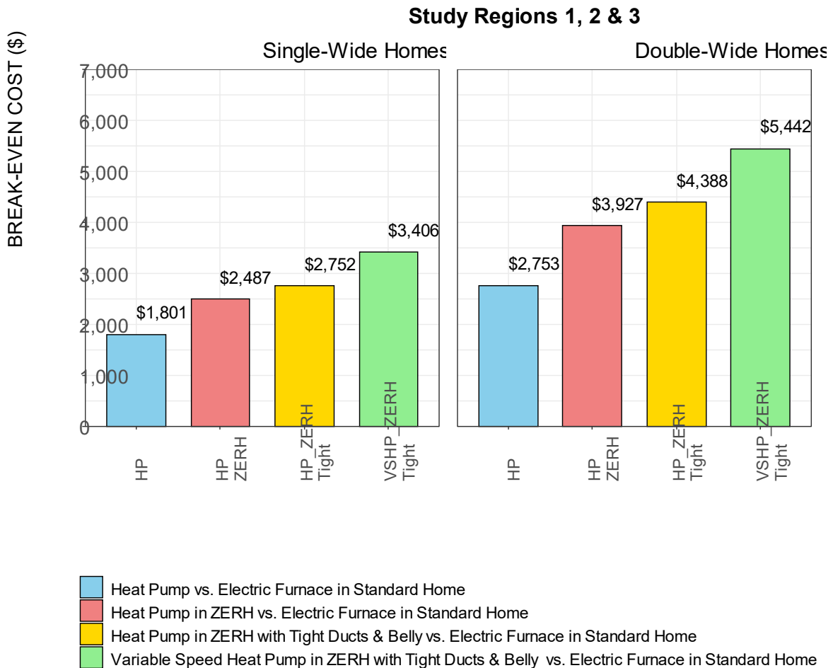
EX-4 Incremental first cost for various measure packages showing consumer cost savings. Weighted average of regions 1, 2 and 3 (warm climates).
