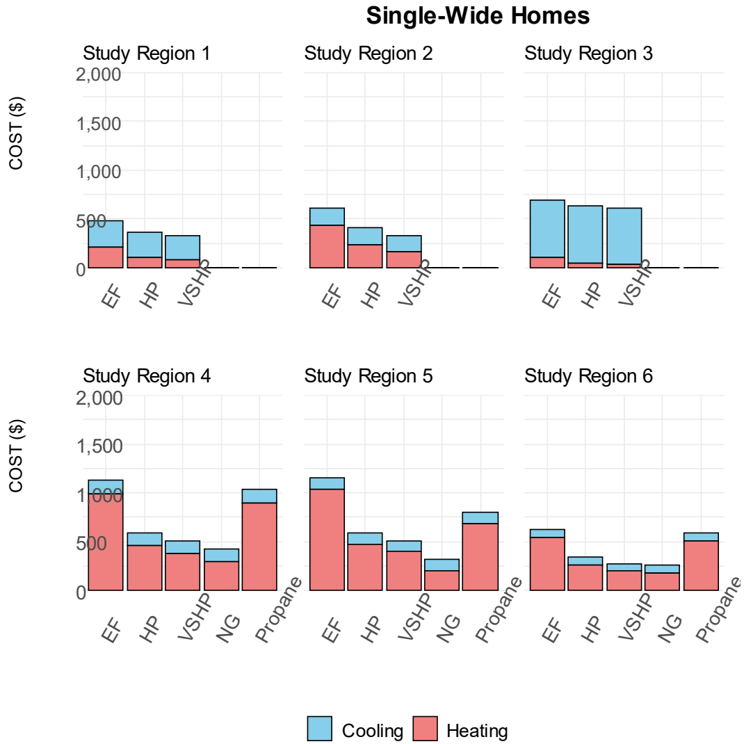
Figure 28. Estimated annual heating and cooling costs for baseline envelope with selected HVAC types, by study region, for single-wide homes.
