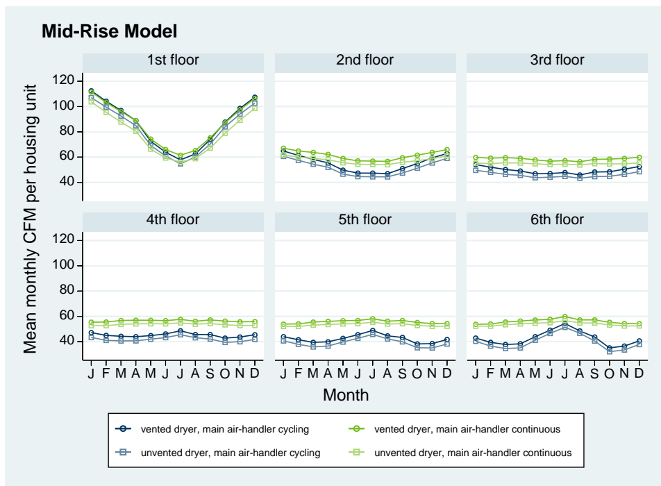
Figure 30. Monthly average CONTAM-modeled air exchange for the mid-rise model, by modeled condition and level.
