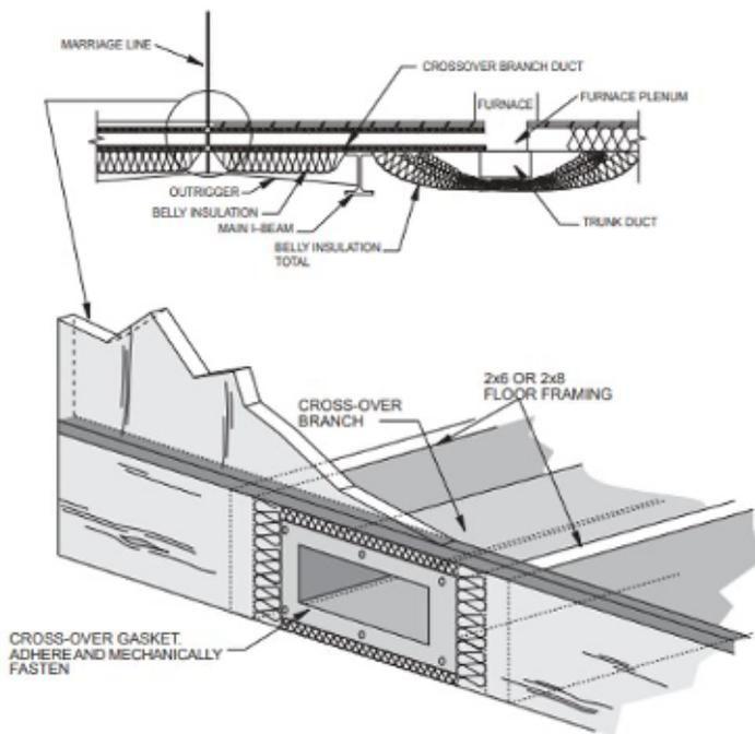
Figure 1: Example through-the-rim crossover-duct design.
