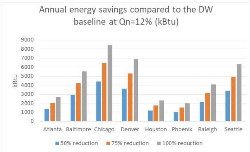
Figure 14. Energy savings (percent) associated with 50%, 75% and 100% reduction in duct leakage for a double-wide home with an electric furnace and central A/C, by city.
