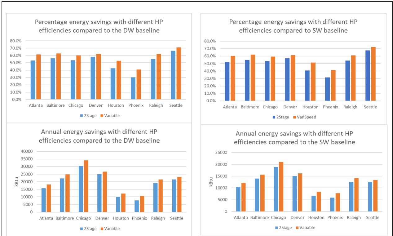
Figure 12. Two-stage and variable speed heat pump savings relative to an electric furnace with conventional central A/C under the efficient baseline assumptions.
