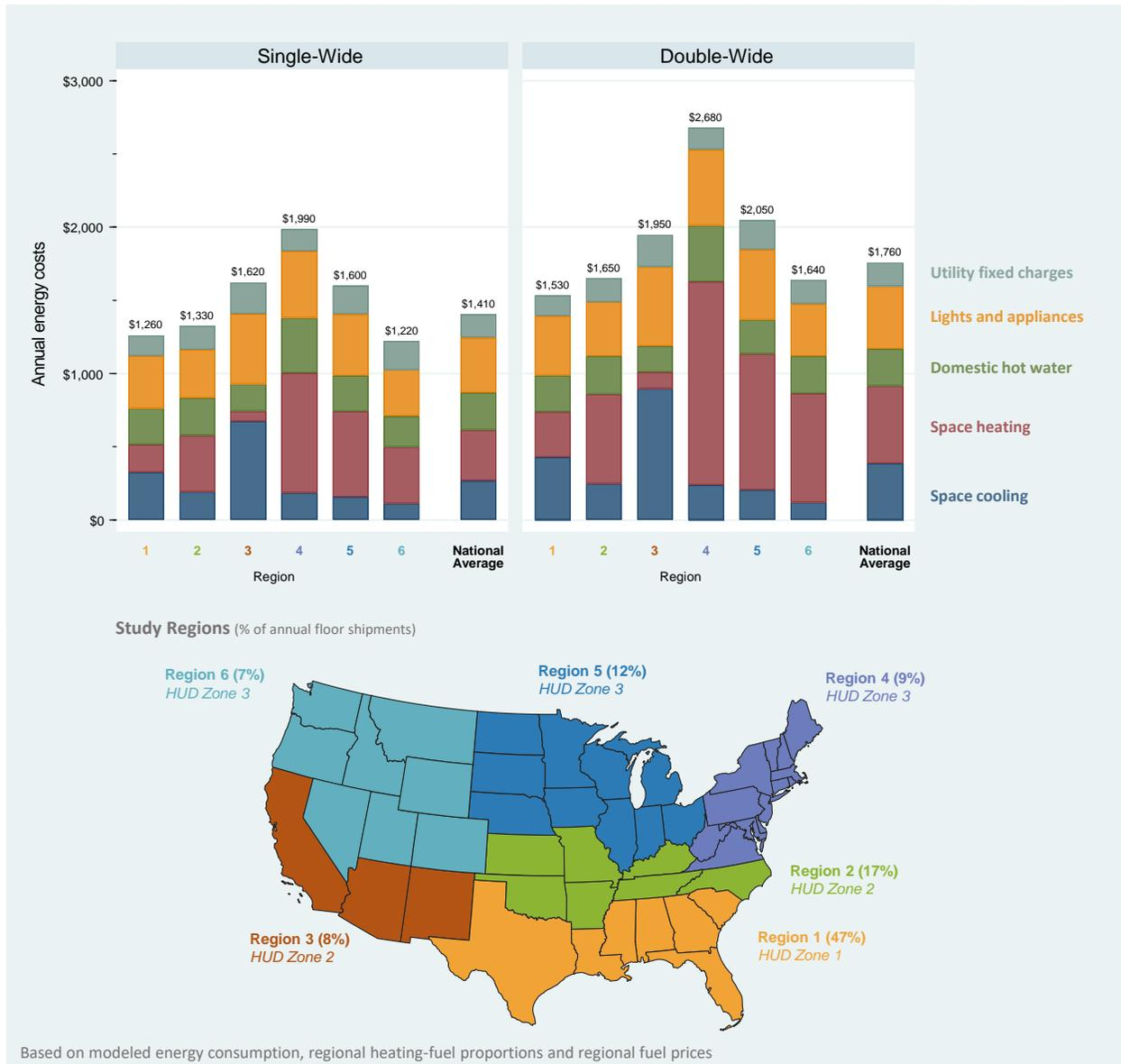
Figure 19. Estimated heating and cooling costs by type of home and modeled location.
