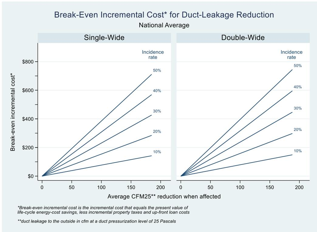
The actual incidence and magnitude of leakage reductions for the innovations is difficult to know. But given ranges for these, the results above can be used to roughly bound the supportable incremental cost for innovations that seek to reduce duct leakage. Table 20 shows national-average ranges for energy-cost savings and break-even incremental costs for what we consider to be plausible ranges of incidence and magnitude for the innovations that seek to reduce duct-leakage.
