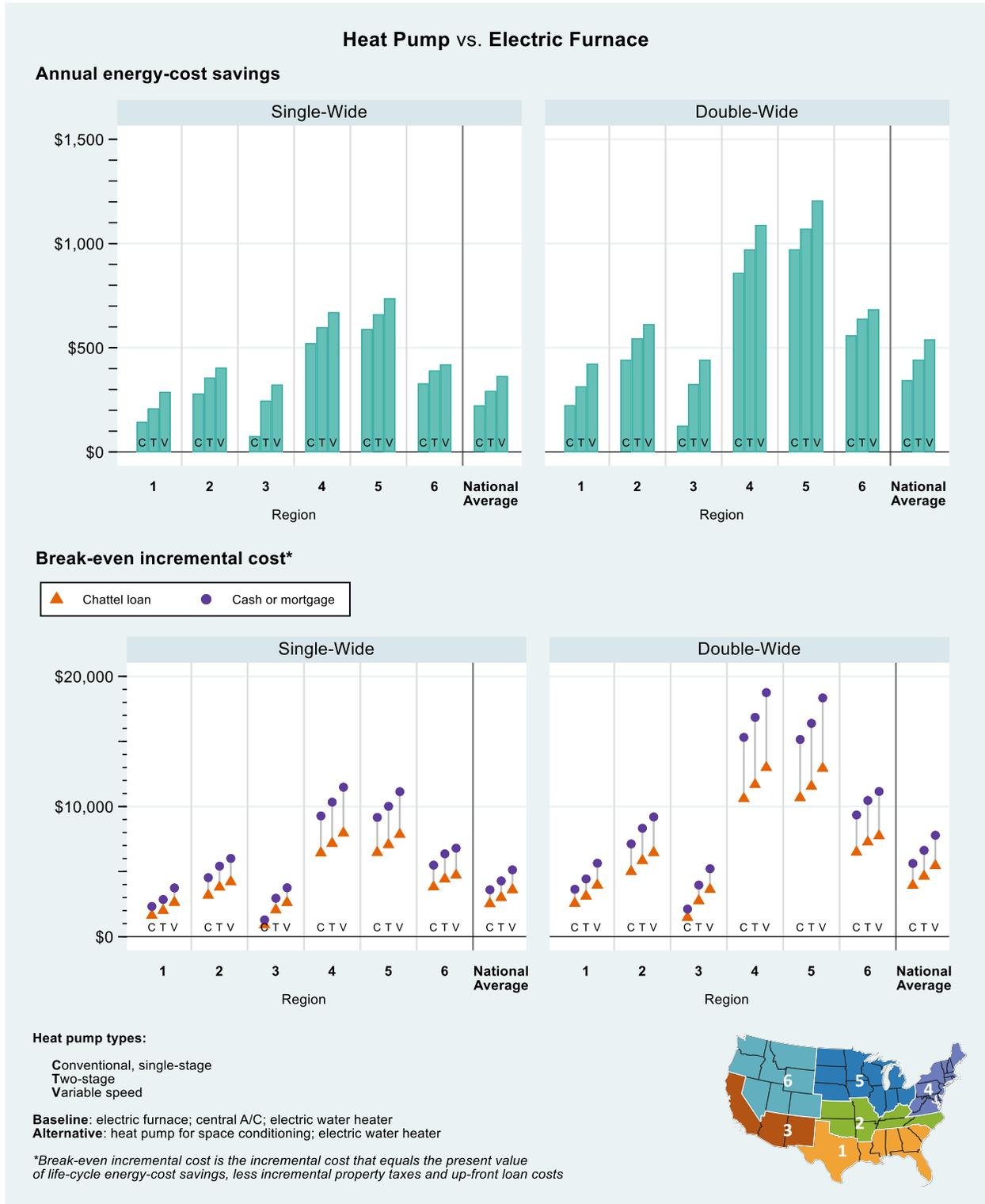
Figure 23. Energy-cost savings and break-even incremental cost for three types of heat pumps compared to a propane furnace with central A/C, by home type and region.
