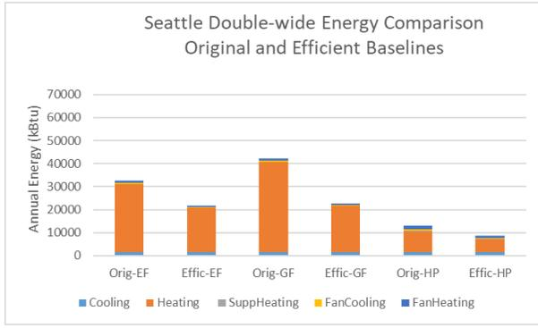
Table 7. Efficient-baseline total HVAC energy use compared to the original baseline, by city and mechanical-system type.
