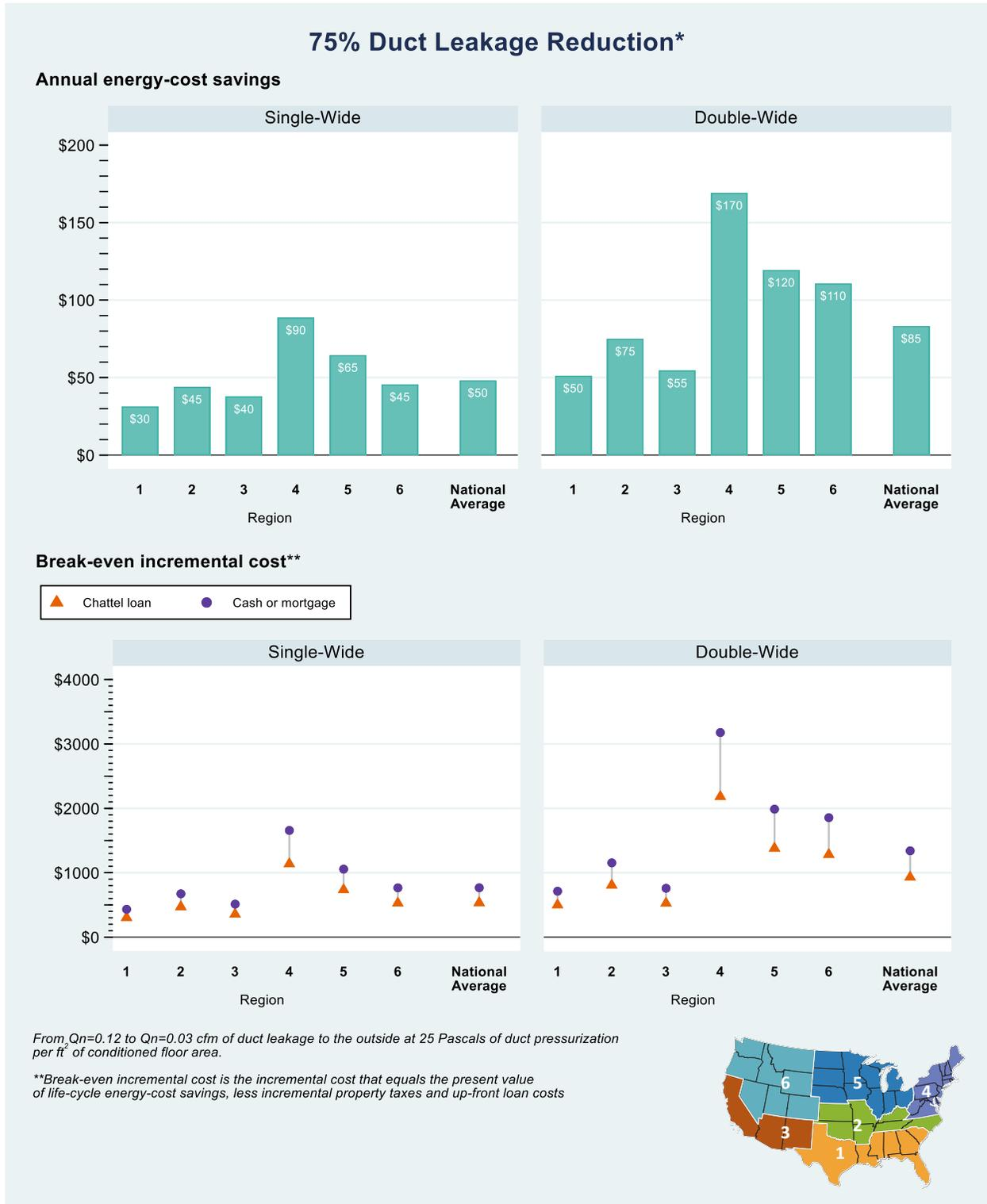
Figure 29. National average break-even incremental cost for resolving duct-leakage issues, by home type.
