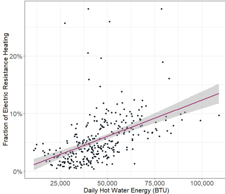
Figure 17. Fraction of electric resistance energy vs. daily hot water energy with regression line for site 03, calculated by day.
