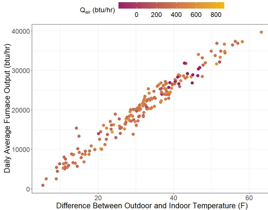
Figure 18. Site 8 daily furnace energy by the average temperature difference. The color gradient shows the amount of  $Q_{air}$  energy extracted from the house on that day.
