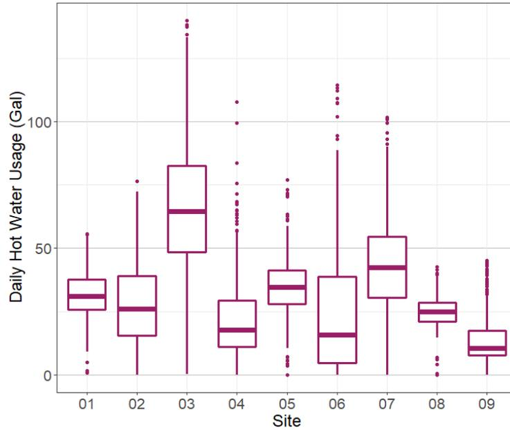
Figure 7. Distribution of daily hot water use by site. The boxes represent the 25<sup>th</sup> to 75<sup>th</sup> percentiles, and the heavy line is the median value. For readability, plots exclude the highest one percent of observations. Days of no hot water use are included.
