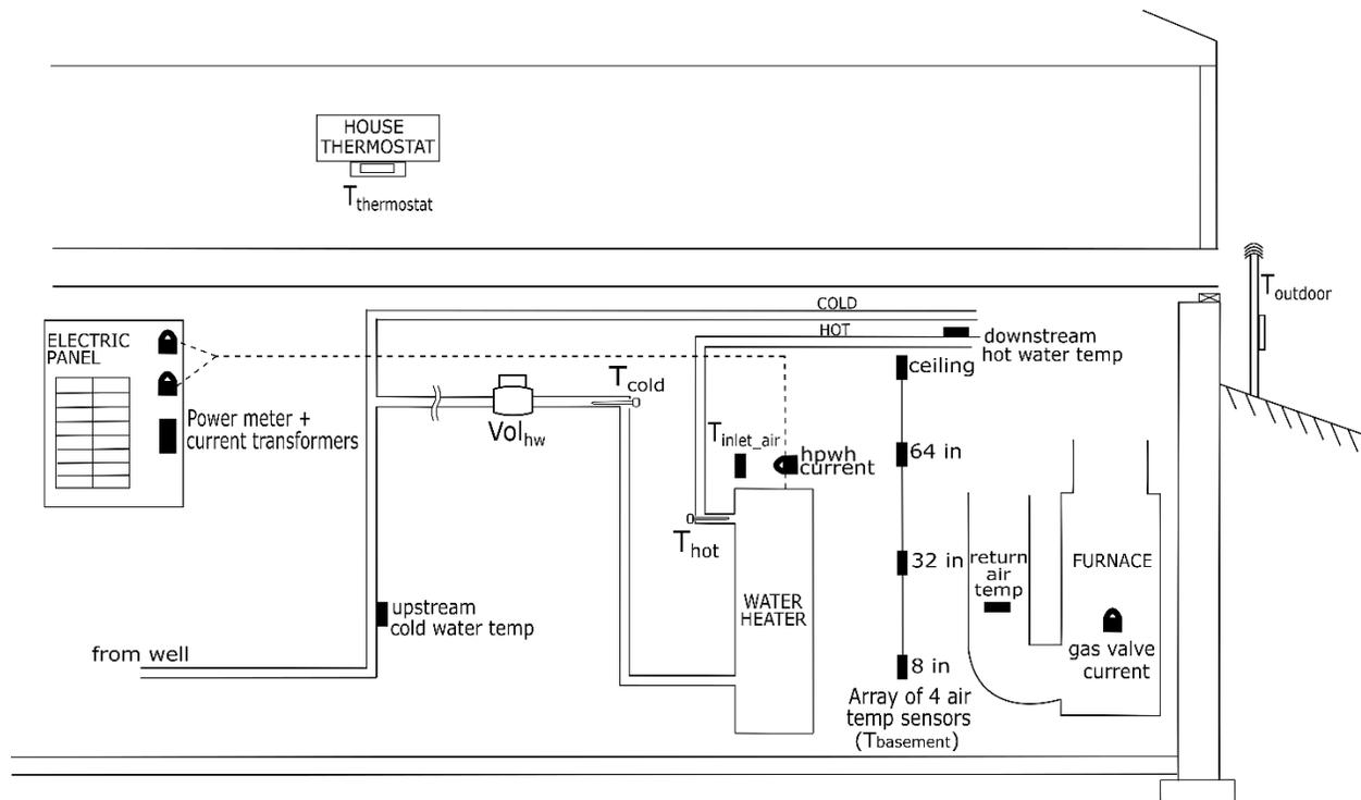
Figure 3. Monitoring system component positions.
