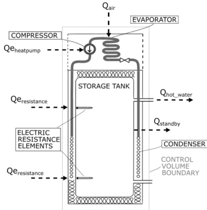
Figure 29. Energy entering and leaving a heat pump water heater, with control volume.
