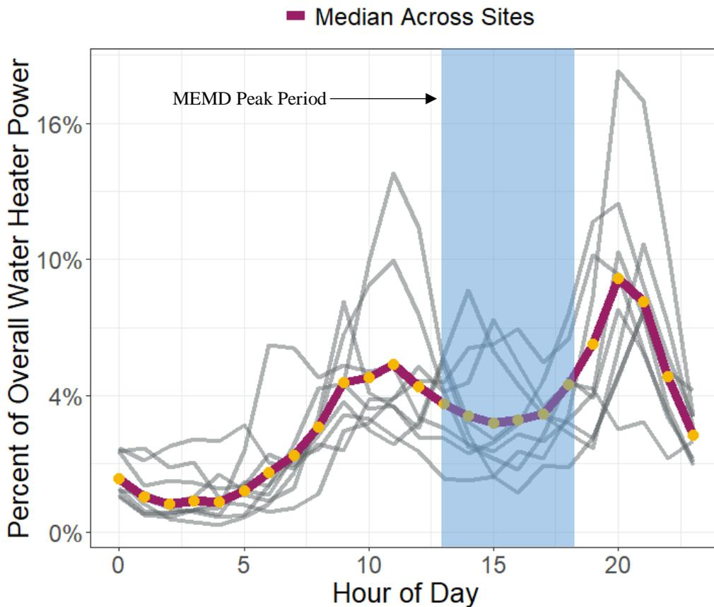
Figure 28. Hourly loads by site (in grey) and median across sites. Shading shows the MEMD-defined coincident peak period.<sup>31</sup>
