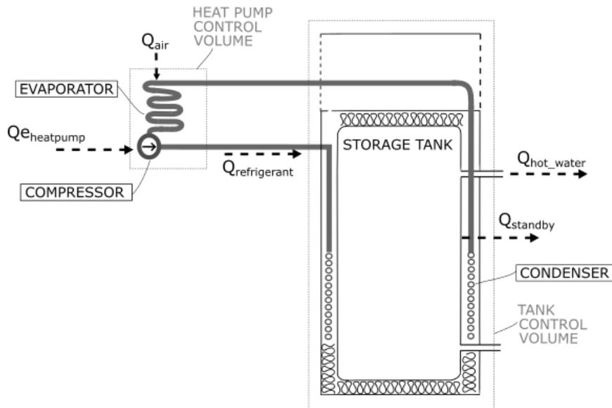
Figure 6. Energy entering and leaving the heat pump control volume, used in COP calculation.
