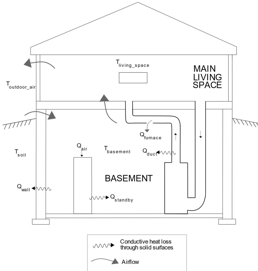
Figure 31. Major mechanisms influencing basement temperature and coupling with main living space.
