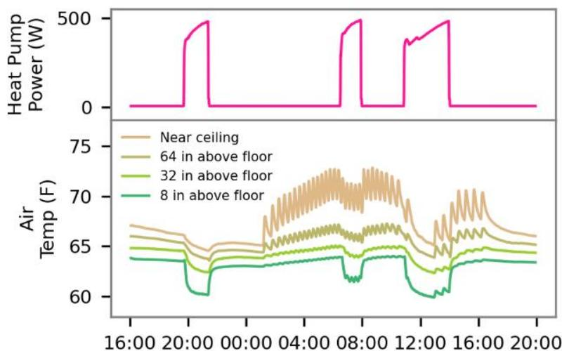
Figure 19. Basement temperature trends during heat pump and furnace cycling.
