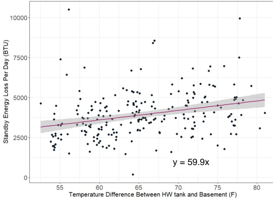
Figure 15. Standby loss vs tank - basement temperature difference for all sites, with regression line.
