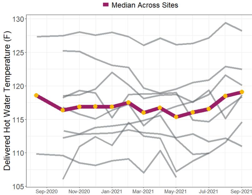
Figure 10. Average monthly hot water temperature by site over the monitoring period. Hot and cold water temperatures are weighted by flow.
