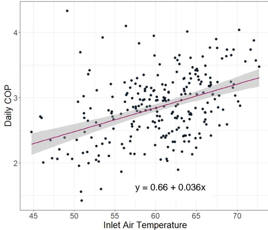
Figure 16. COP vs. inlet air temperature with regression line for site 04, calculated by day. The slope of 0.036 translates to a 1-unit increase in COP for a 28 °F increase in inlet air temperature.
